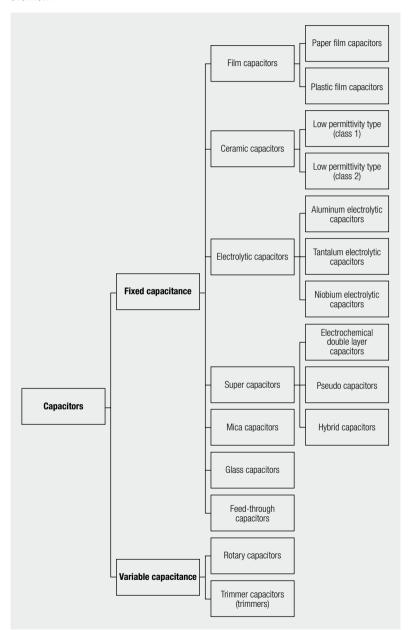
Fig. 3.1: Overview of existing capacitor types
