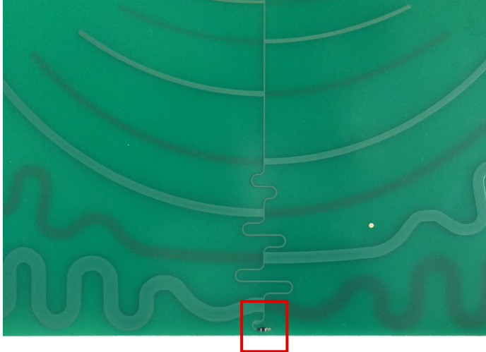
Figure 22: PCB of an LPDA with WE-CBF HF (742862160).
