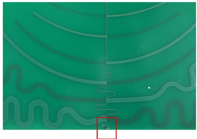
Figure 22: PCB of an LPDA with WE-CBF HF ( 742862160 ).
