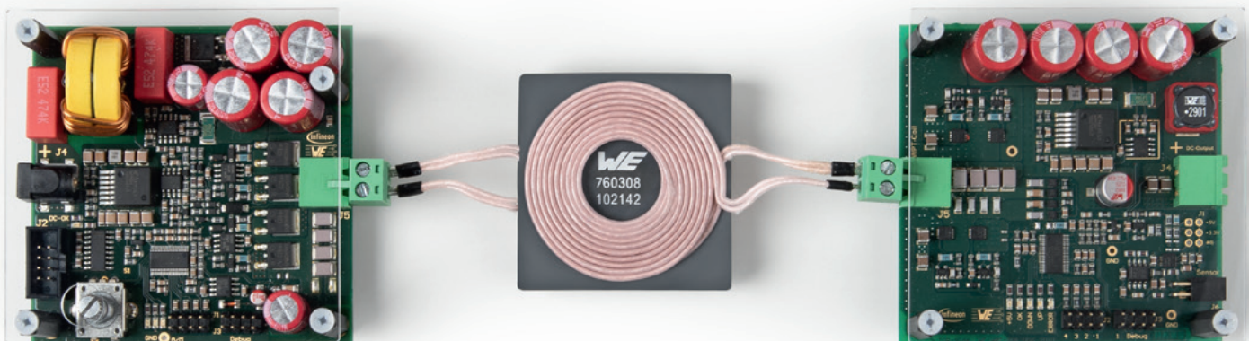
Figure 1: Wireless power transfer system with transmitter board, coils and receiver board.
