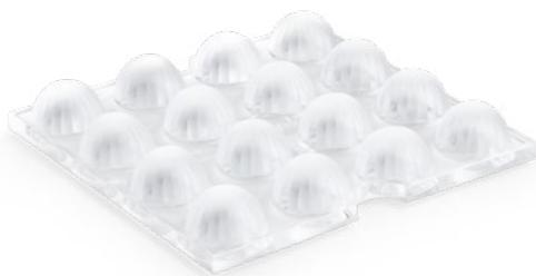
The LEDiL® Stradella multi-lens was designed, so that every LED on its own gives the optimal light yield. Therefore inside the lens the LED light beam is steered. The angle of radiation is 60° for the Horticulture Panel setup. Using a M3 screw and M3 screw nut to counter the screw the lense can be mounted to the Horticulture Panel.
