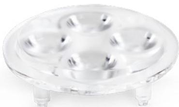
The LEDiL® PMMA multi-lens was designed, so that every LED on its own gives the optimal light yield. The LED light beam is focused and directed inside the lens. The angle of radiation is either 30° or 55° for the RGBW Panel setup. Via pin by pin adhesive bonding the lense can be fastened to the RGBW Panel.
