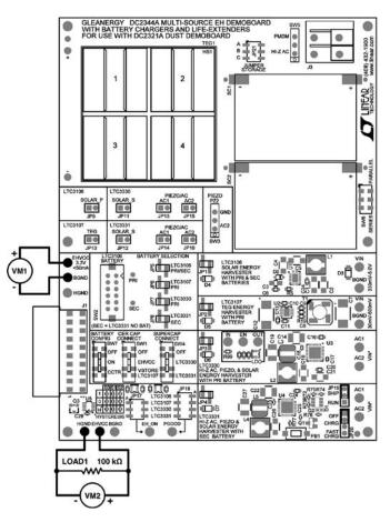
Figure 5. Setup for General DC2344A Test Procedure
