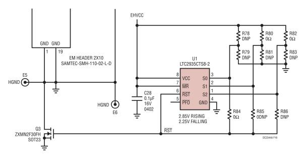
Figure 16. Schematic of LTC2935-2 Low-Power Supervisor and HGND Switching Circuit
