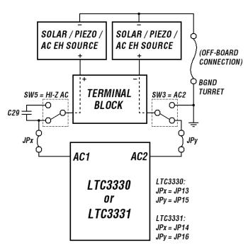
Figure 26. Dual-Source Configuration Routing
