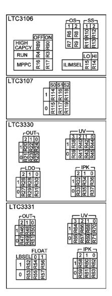
Figure 20b. Back  $0\Omega$  Resistor Jumpers for Tables 10-16
