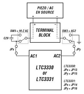
Figure 25. Full-Wave Rectifier Configuration Routing
