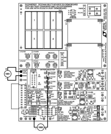
Figure 6. Setup for DC2344A Test Procedure with LTC3107
