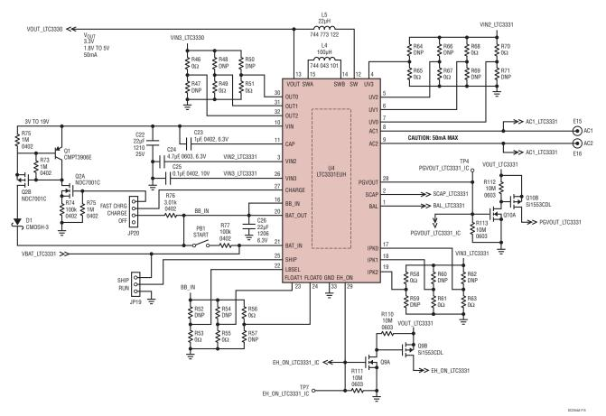
Figure 15. Schematic of LTC3331 Hi-Z AC, Piezoelectric, & Solar Energy Harvesting Power Supply
