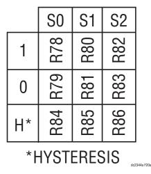
Figure 20a. Front 0 $\Omega$  Resistor Jumpers for Table 9
