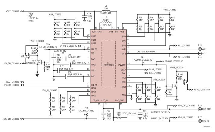
Figure 14. Schematic of LTC3330 Hi-Z AC, Piezoelectric, & Solar Energy Harvesting Power Supply
