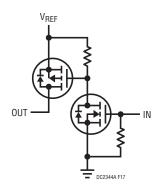
Figure 17. Simple Signal Buffer/Level Translator Circuit
