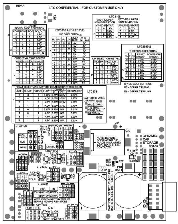
Figure 4. DC2344A Bottom Assembly Drawing
