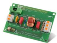
Multiple Line Filter 250 V, with overvoltage protection Order Code.: 7449984
