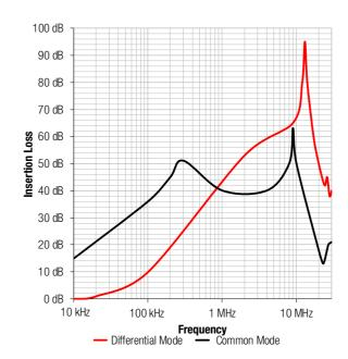
Measured example with Cx: WCAP-FTX2 150 nF CMC: WE-CMB S 10mH Cv: WCAP-CSSA MLCC 2.2 nF
