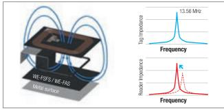
Shielded NFC-RFID Communication. WE-FSFS/WE-FAS protect communication by concentrating the magnetic field. Frequency swift due to close Metal surfaces is prevented. **Applications**
