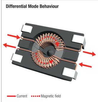
In opposition to the common mode behaviour, the differential mode component of the signal will see almost no impedance in the choke, this phenomenon could be explained with the magnetic field compensation inside the core. If the core is not magnetized, then no inductance will appear in the line.
