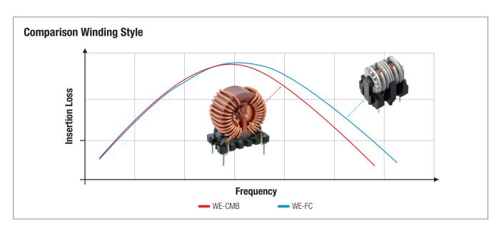
A division of the winding space in separate chambers (see WE-FC, 2 chambers on each winding) reduces the intrawinding capacitance increasing the bandwith of the choke. The current capabilities will be reduced due to the smaller winding space.
