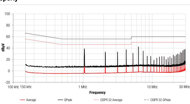
Figure 10: EMC measurement with input filter and aluminum polymer capacitor C1
