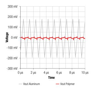
Figure 13: Measurement of ripple voltage when using the aluminum polymer capacitor at the output
