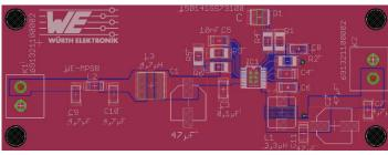
Figure 4: Layout of the buck converter
