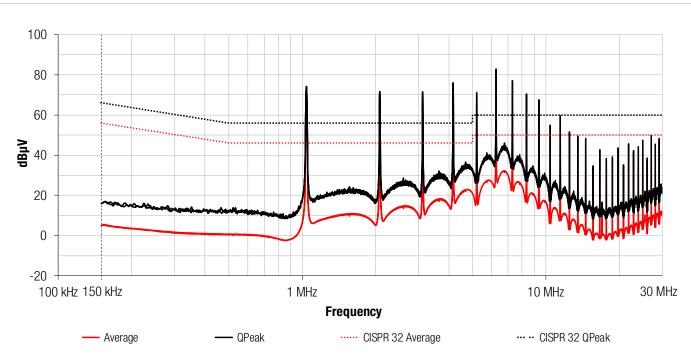
Figure 8: EMC measurement with an aluminum polymer capacitor as input capacitor C1
