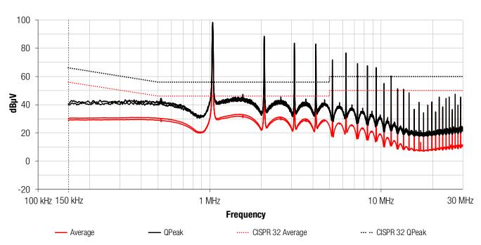
Figure 6: First EMC measurement with an aluminum electrolytic capacitor as C1
