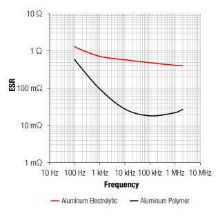
Figure 12: Comparison of the ESR of the aluminum and aluminum polymer capacitor
