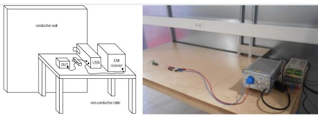
Figure 5: Setup of the EMC measurement according to CISPR 35
