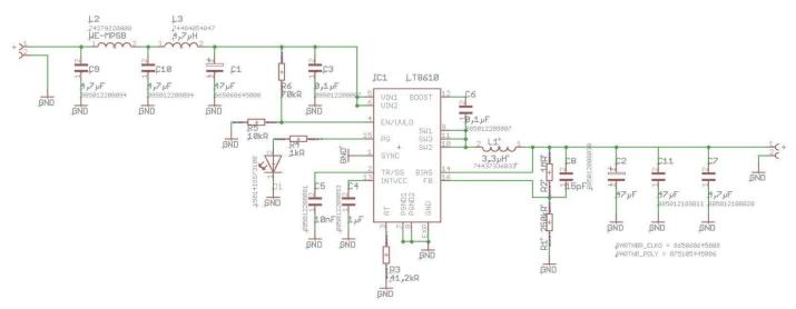
Figure 3: Schematic of the buck converter
