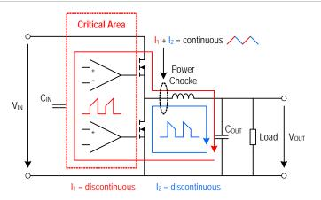
Figure 2: Principle of a buck converter
