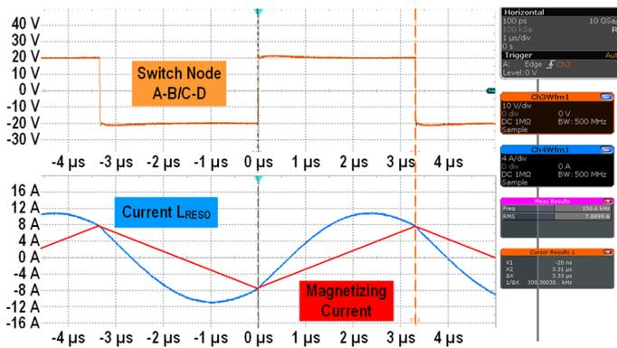
**Figure 8: Switching frequency and magnetising current**
