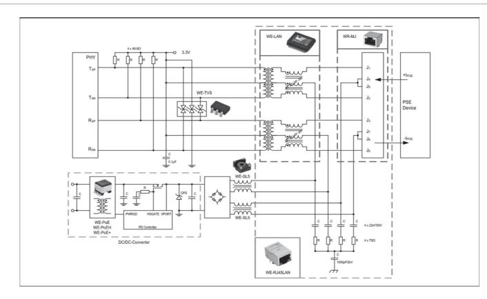
A connection between LAN and Power over Ethernet (PoE) follows the structure as shown in the picture. The Ethernet signals are routed through the cable to the PHY chip whereas the PoE current is transmitted over the same cable and will flow towards the DC/DC converter.
