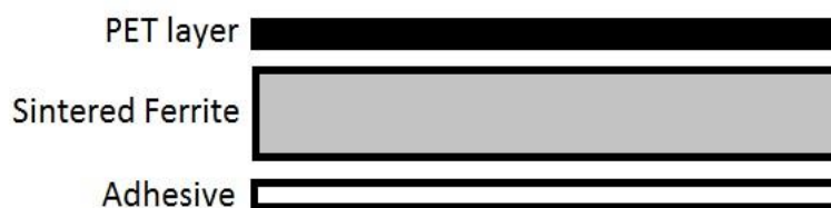
Figure 2: Construction of WE-FSFS sheet
