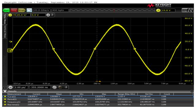
Figure 4: Voltage at the transmitter coil (not referenced to circuit GND; Vin = 20 V / Pout = 100 W)
