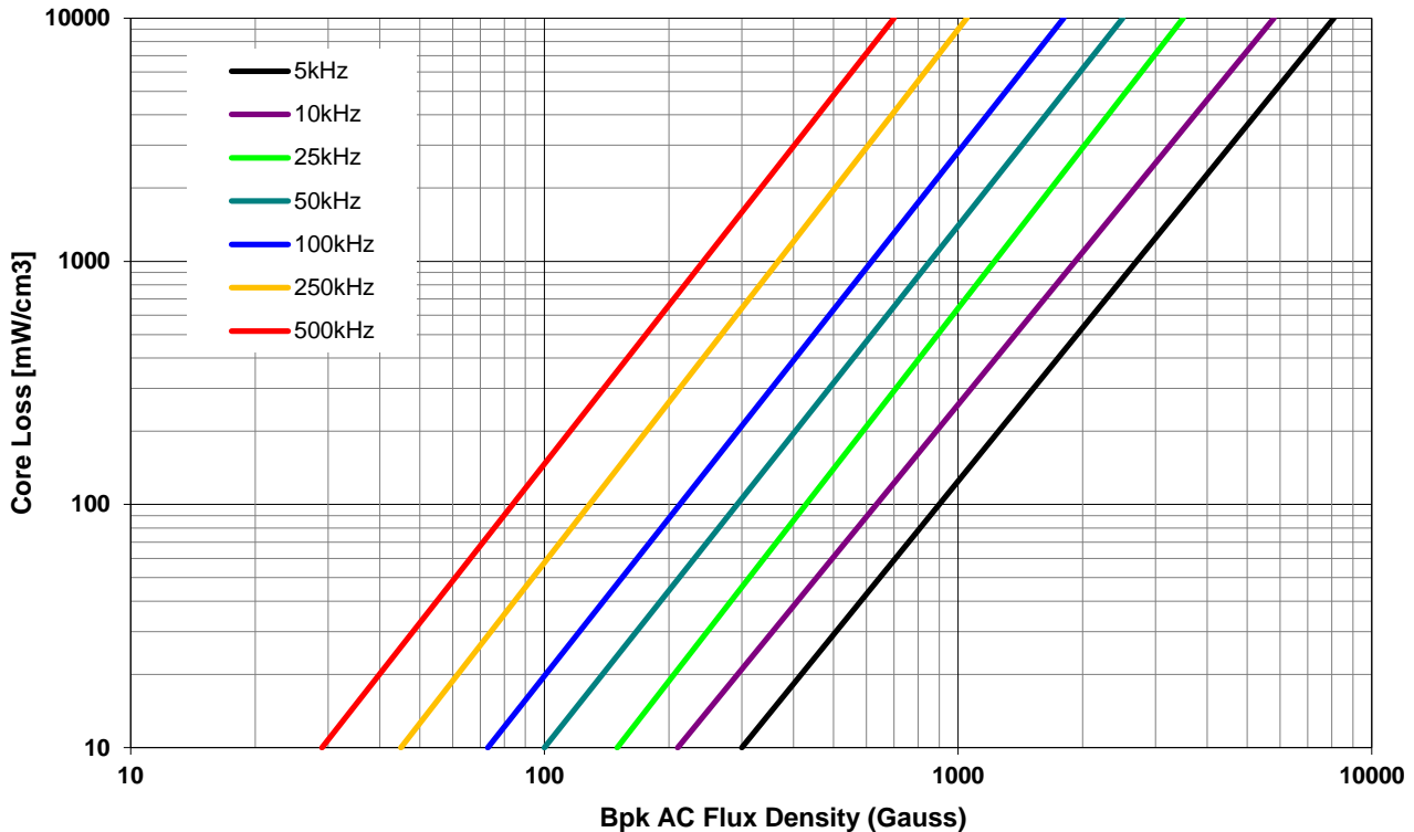
Figure 2: Core Loss graph plotted against peak flux density at different frequencies
