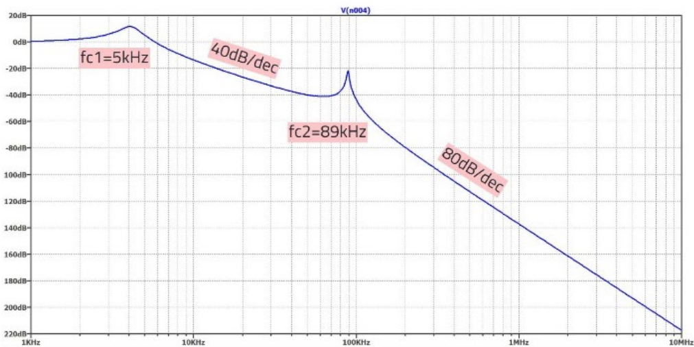
Figure 48: The two-stage filter attenuation behavior.
