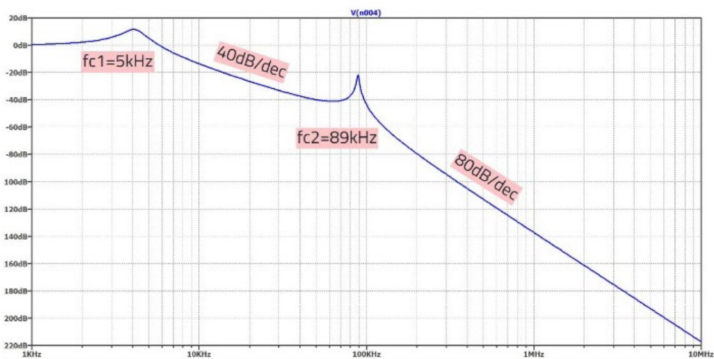
Figure 48: The two-stage filter attenuation behavior.
