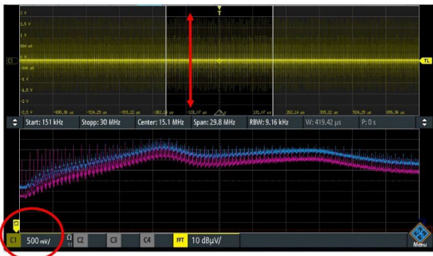
Figure 3: The vertical resolution or scale of the channel is optimized, to obtain the highest sensitivity.
