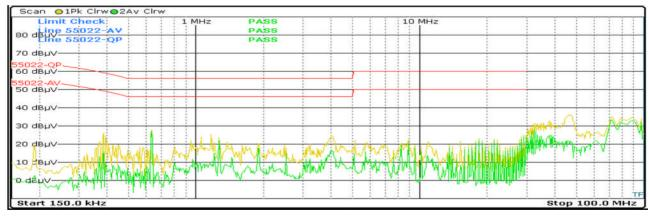
Figure 29: Measurement of the interference voltage of Design (2) at the output of the boost converter with filter  $(15 \mu H / 10 \mu F / Stroko 5 mH)$
