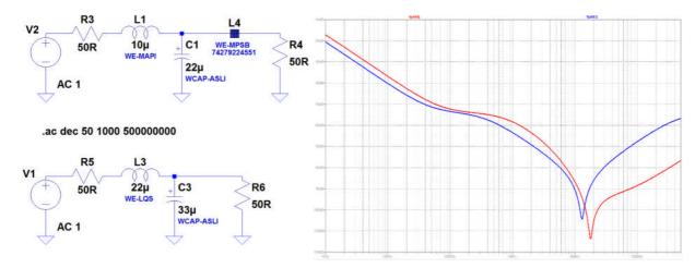
Figure 8: Simulated (LT Spice) suppression of a pure LC filter (22 $\mu$ H + 33 $\mu$ F blue) and a T filter (10 $\mu$ H + 22 $\mu$ F + MPSB 74279224551 red) in a 50 $\Omega$  system (1kHz - 500MHz).
