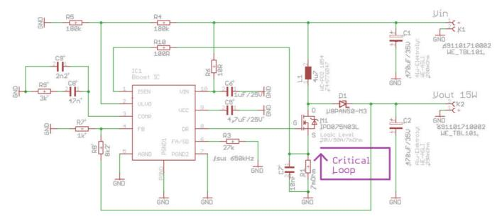
Figure 13: Circuit diagram of a critical design (Design 1) with  $U_{ln} = 9 \text{ V}$ ,  $U_{out} = 12 \text{ V}$ ,  $I_{out} = 1.25 \text{ A}$ ,  $I_{sw} = 650 \text{ kHz}$
