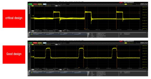
Figure 35: Measurement of the drain-source voltage at the MOSFET
