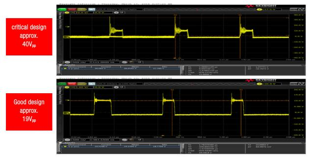
Figure 36: Measurement of the voltage over the Schottky diode
