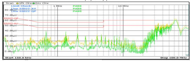
Figure 21: Measurement of the interference voltage of Design (1) at the output of the boost converter with LC filter (15 μH / 10 μF)
