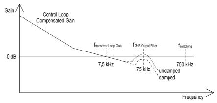
Figure. 12: Setting of the various frequencies as a factor of the circuitry and switching frequency
