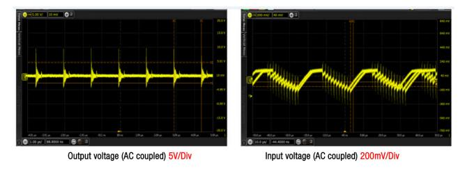
Figure 19: Measurement of the interferences in the time domain of Design (1) at the input and output of the boost converter w/o filter
