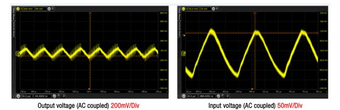
Fig. 28: Measurement of the interferences in the time domain of Design (2) at the input and output of the boost converter w/o filter
