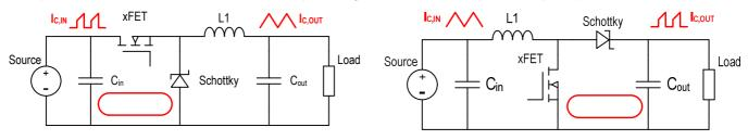
Figure 5: critical current loop buck converter
