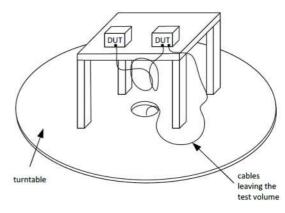
Figure 1: Test set-up for interfering voltage
