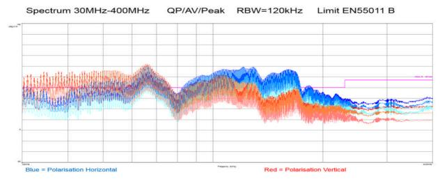
Fig. 25: Measurement of Design (1) w/o decoupling filters
