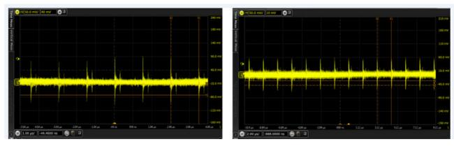
Output voltage (AC coupled) 50mV/Div
