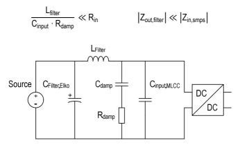
Figure 10: Measures for filter suppression: SMD resistor in series with a capacitor
