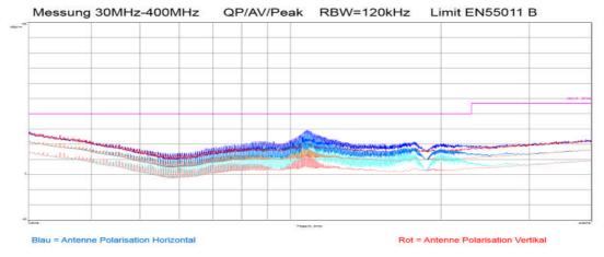
Figure 32: Measurement of design (2) with decoupling filters
