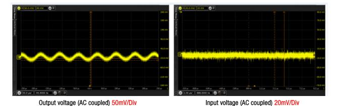
Fig. 31: Measurement of the interferences in the time domain of Design (2) at the input and output of the boost converter with filter
