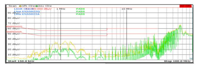
Figure 22: Measurement of the interference voltage of Design (1) at the input of the boost converter with LC filter (15 µH / 10 µF)
