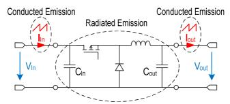
Figure 4: Potential sources for conducted and radiated emission
