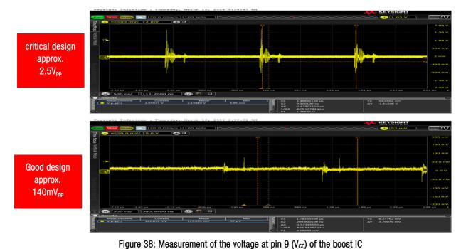
rigule 30. Measurement of the voltage at pin 9 (VCC) of the boost to
