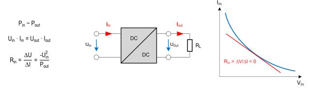
Fig. 9: Since the output remains constant even in the case of a drop in the input voltage, it is logical that the input current must rise.
