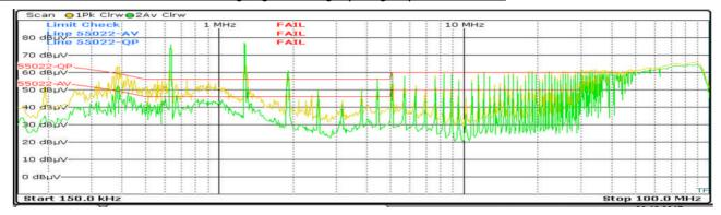
Figure 26: Measurement of the interference voltage of Design (2) at the output of the boost converter w/o filter
