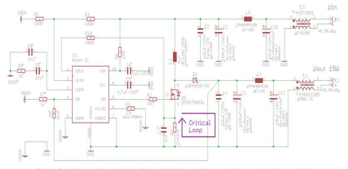
Fig. 15: Circuit diagram of a good design (Design 2) with Uin = 9 V, Uout = 12 V, lout = 1.25 A, fsw = 650 kHz
