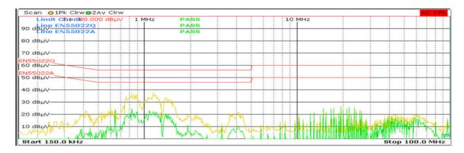
Figure 30: Measurement of the interference voltage of Design (2) at the input of the boost converter with filter (15  $\mu$ H / 10  $\mu$ F / Stroko 5  $\mu$ H)
