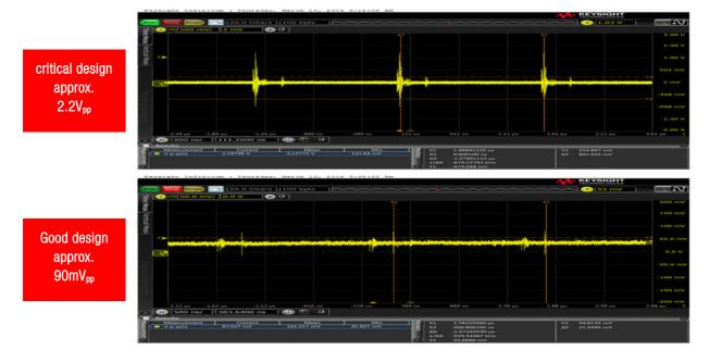
Figure 37: Measurement of the voltage at pin 10 (V<sub>IN</sub>) of the boost IC
