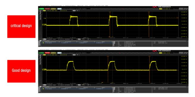
Figure 34: Measurement of the gate-source voltage at the MOSFET
