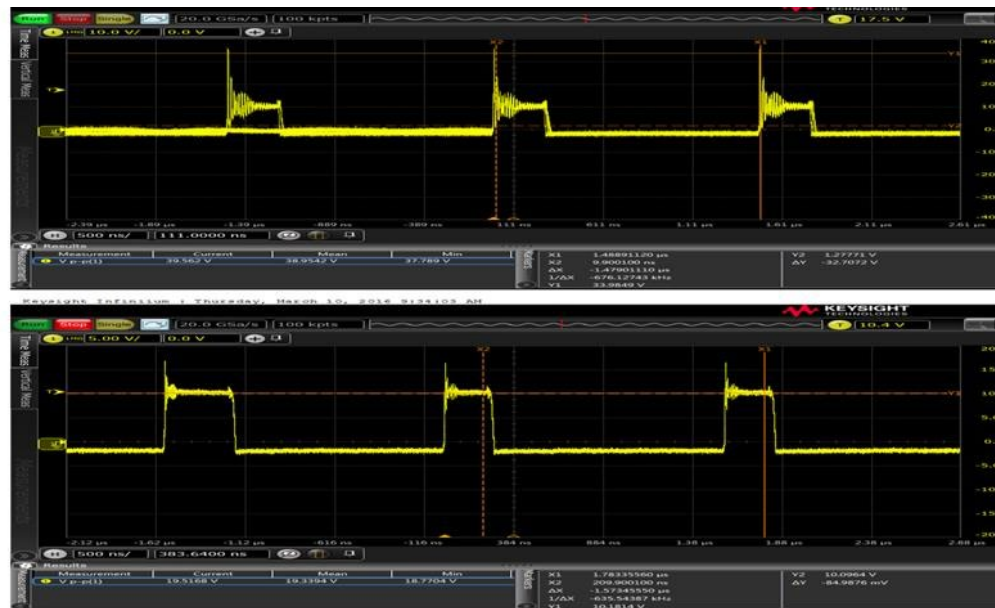
Figure 36: Measurement of the voltage over the Schottky diode.
