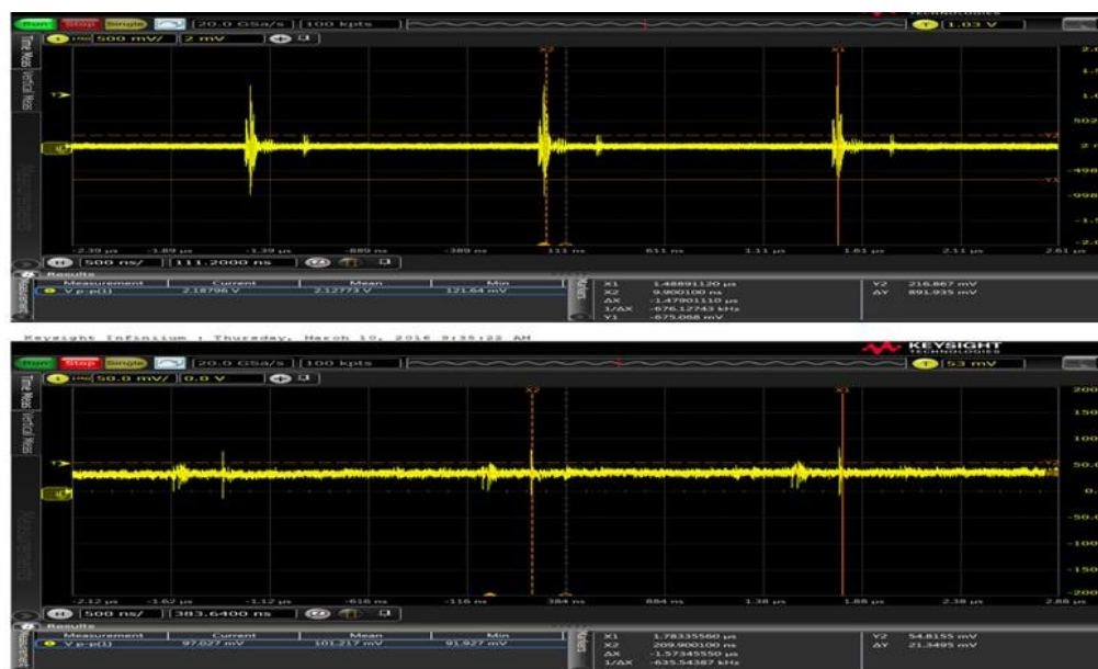
Figure 37: Measurement of the voltage at pin 10 (V IN ) of the boost IC
