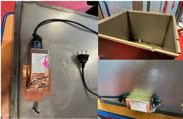
Figure 9: Shielding box to reduce the interference from the auxiliary equipment. The 230 V<sub>AC</sub> supply is filtered into the box using a two-stage filter at the feedthrough. Shielded cables are connected to the package ground at the shielding feedthrough, and the cover is RF sealed to prevent electromagnetic radiation via openings.
