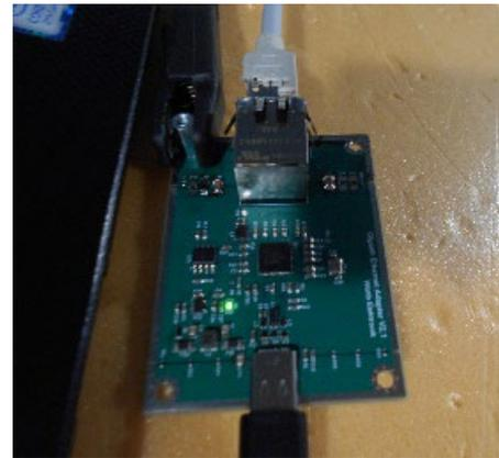
Figure 35: Test setup for direct surge coupling into the cable shield with 2 Ω generator impedance. Surge decoupling by means of an alligator clip and metal bolt on the level of the Ethernet jack – in the picture above left
