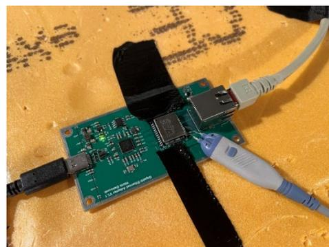
Figure 6: Top: Line code for the Ethernet signal between the transformer and RJ45 jack; Bottom: The measurement setup
