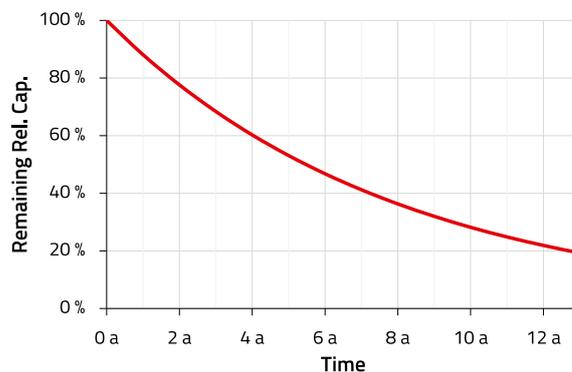
Figure 3: Relative capacitance vs. time for operational profile, given in Table 1.
