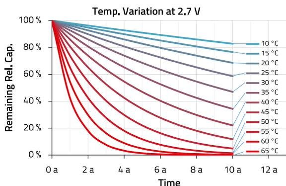
Figure 1: Family of curves calculated for a temperature range from 10°C to 65°C at a constant voltage of 2.7 V.
