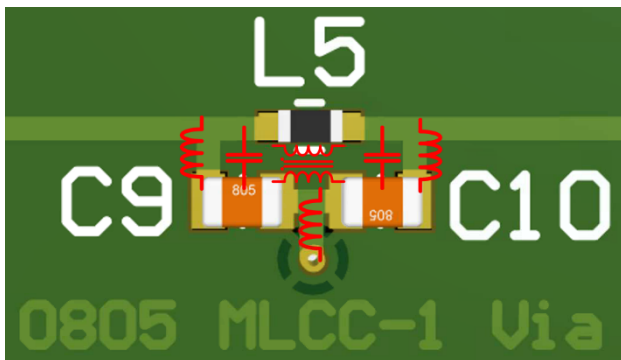
Figure 7: Parasitic inductances and capacitances of the poor layout, which reduce the insertion loss of the filter
