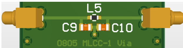
Figure 6: Measuring channel with 0805 MLCC, only 1 via for both GND pads, unnecessary stubs and geometrically unfavorable arrangement compared to the ferrite
