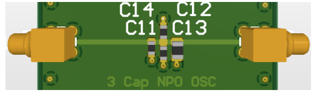
Figure 8: Measuring channel with 3 different capacitance values, but the same dielectric. The fourth MLCC between the labels, was not populated during the tests
