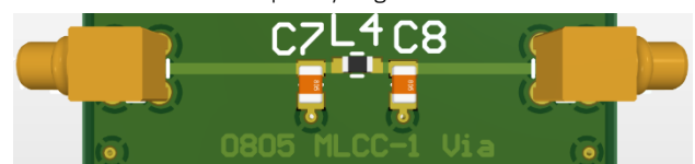
Figure 5: Measuring channel with 0805 MLCC and 1 via each at the GND pad
