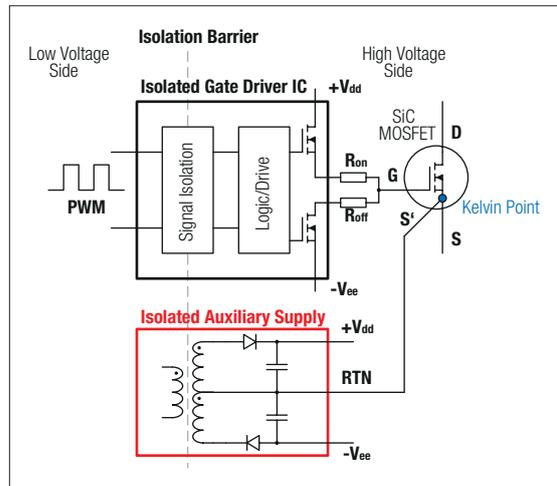
The gate drive IC controller and the auxiliary power supply with bipolar output are configured and connected to the SiC-MOSFET as shown in the image
