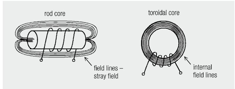
Fig. 2.2: Field line orientation for a rod and toroidal coil
