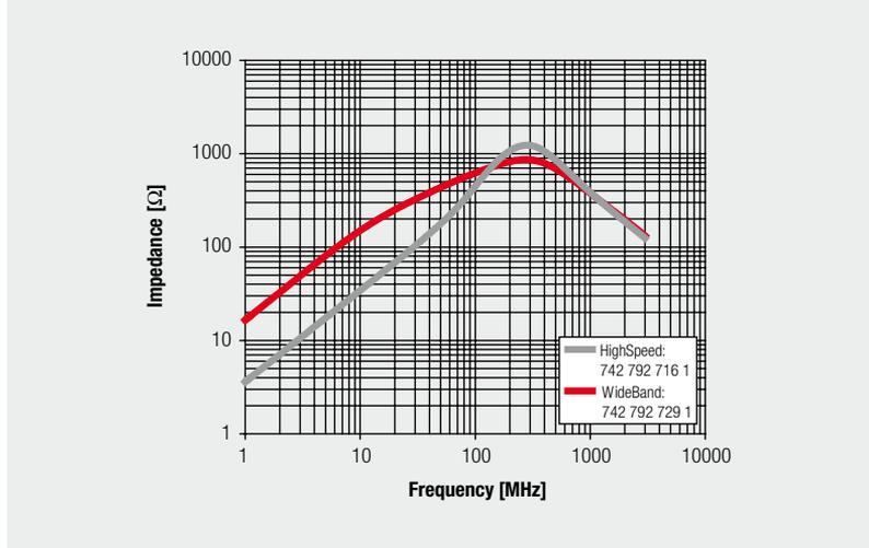
Fig. 2.4: HighSpeed vs. Wideband
