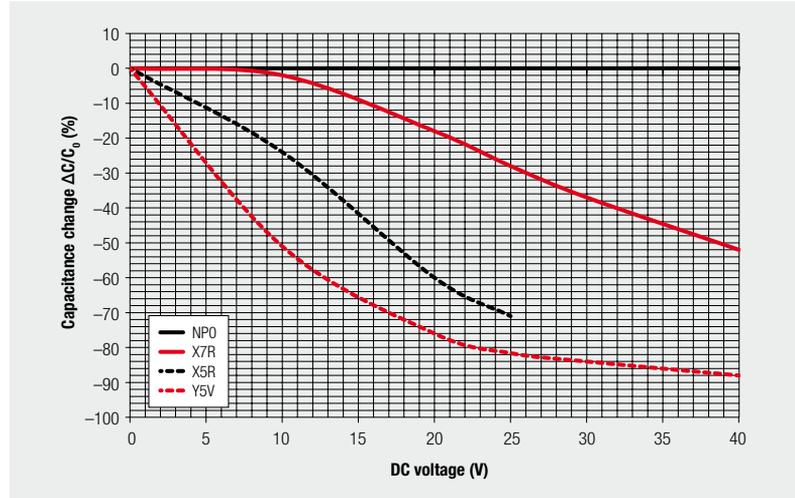
Fig. 2.1: Voltage-dependent capacitance change, example: ceramic capacitors
