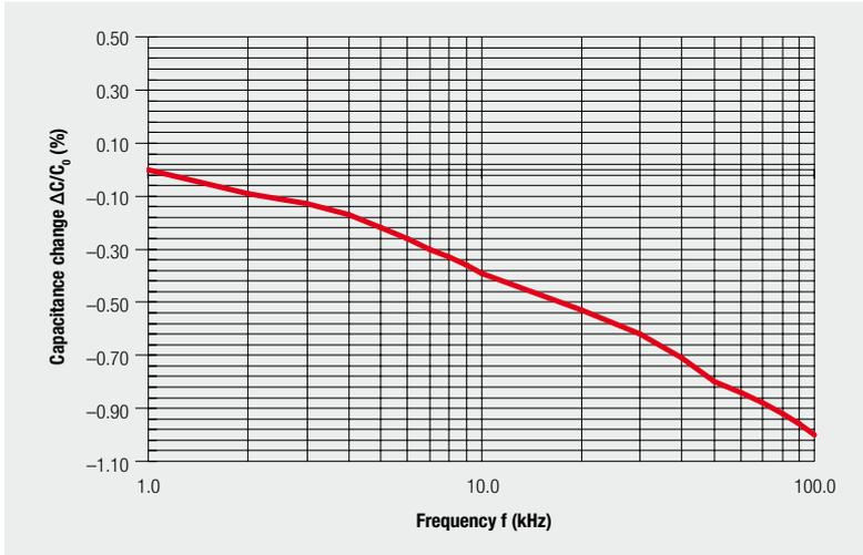
Fig. 2.2: Frequency-dependent capacitance change, example: MKP film capacitor
