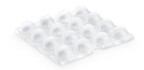
**The LEDIL® Stradella multi-lens** was designed, so that every LED on its own gives the optimal light yield. Therefore inside the lens the LED light beam is steered. The angle of radiation is 60° for the Horticulture Panel setup. Using a M3 screw and M3 screw nut to counter the screw the lense can be mounted to the Horticulture Panel.
