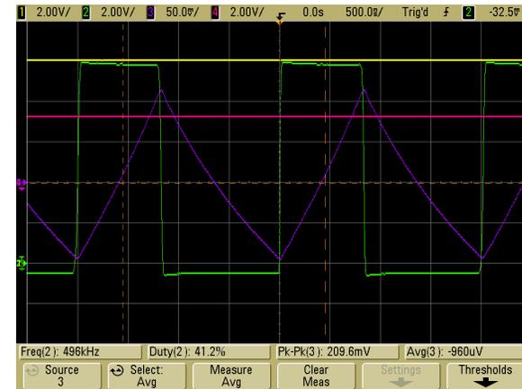
Figure 1.11. Measured waveforms in Test#2 at 1.4A with inductor L1 not heated: ■ input voltage, ■ switching node voltage, ■ output voltage, ■ ripple current
