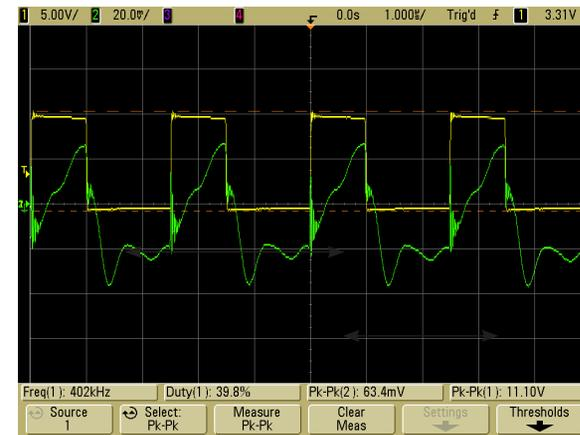
Figure 4.13. Measured waveforms with input filter inductors bypassed
