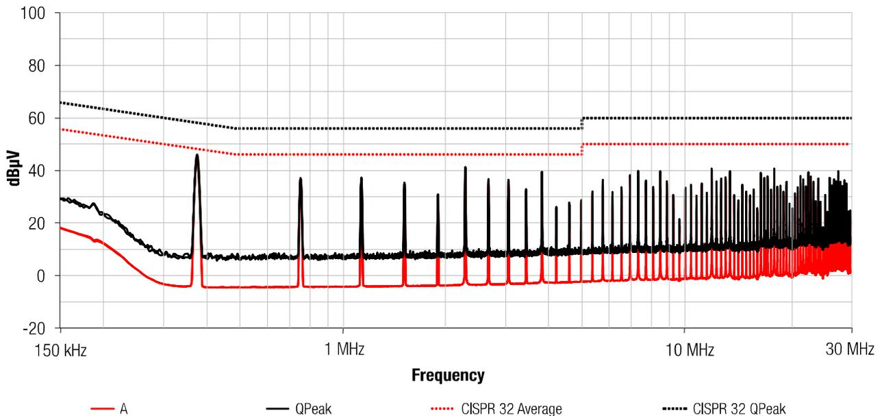
**Figure 22: Radiated interference WITH the input and output filters as specified above. Interference is sufficiently within the specified limit (horizontally and vertically) across the entire measured range.**
