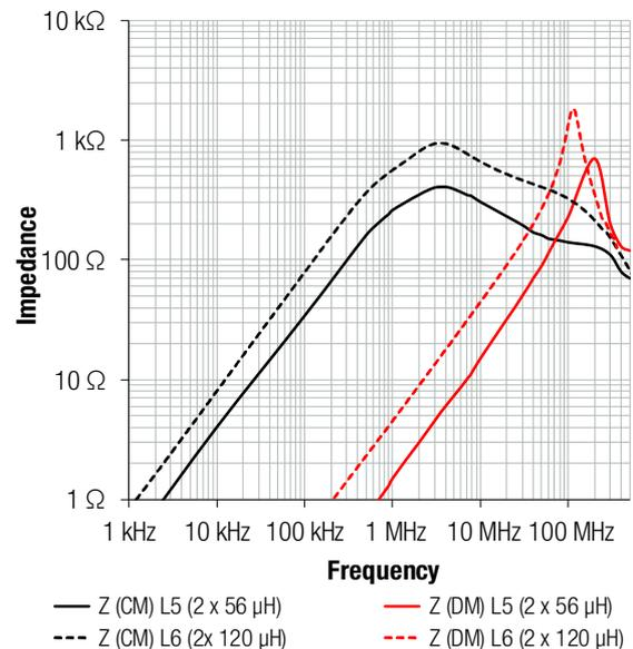
Figure 17: Common mode and differential mode impedance curves of the two WE-UCF current-compensated chokes used
