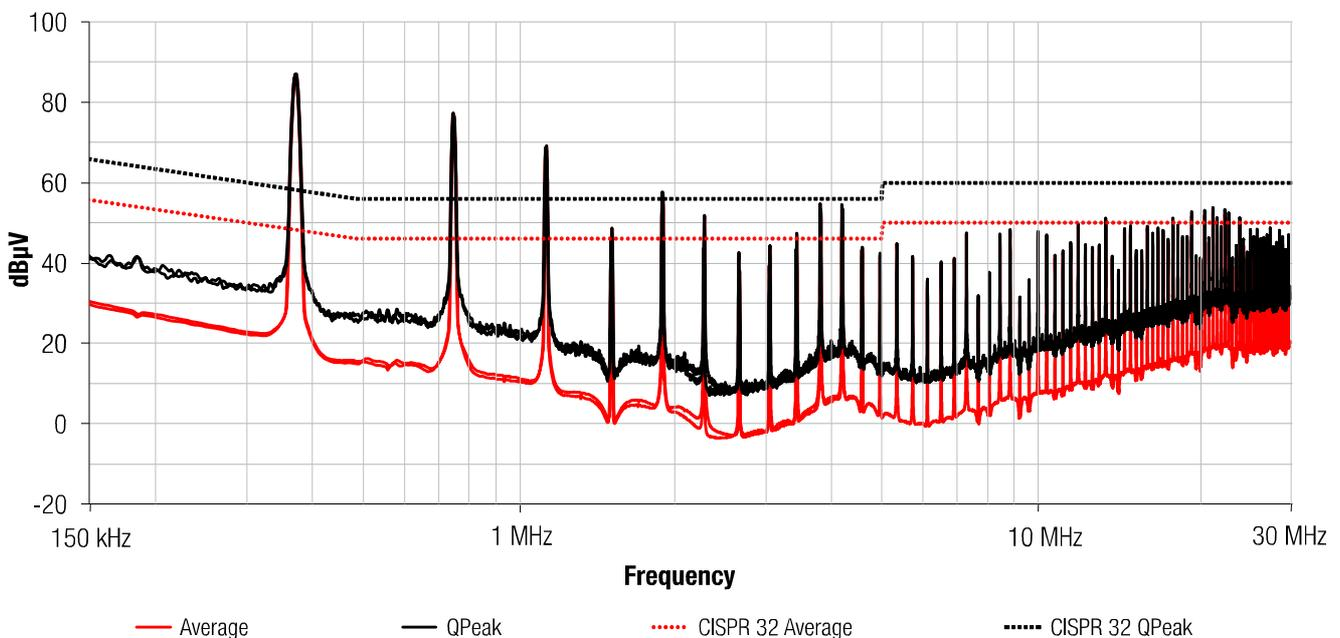
**Figure 13: Measurement of radiated interference WITHOUT input and output filters. The difference between the interference and the limit value is very small at approximately 180MHz, which can cause problems with subsequent measurements. The cause is the fast reverse recovery time of the Schottky recovery current, which stimulates parasitic LC resonance.**
