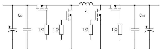
Figure 3: Simplified diagram of the converter power stage.
