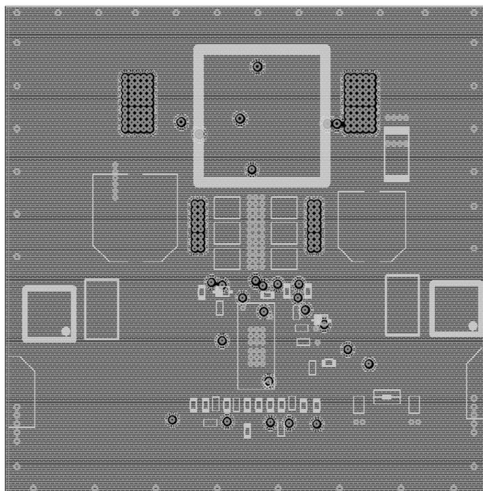
Figure 11: Layout of intermediate layers 2, 4 and 5.
