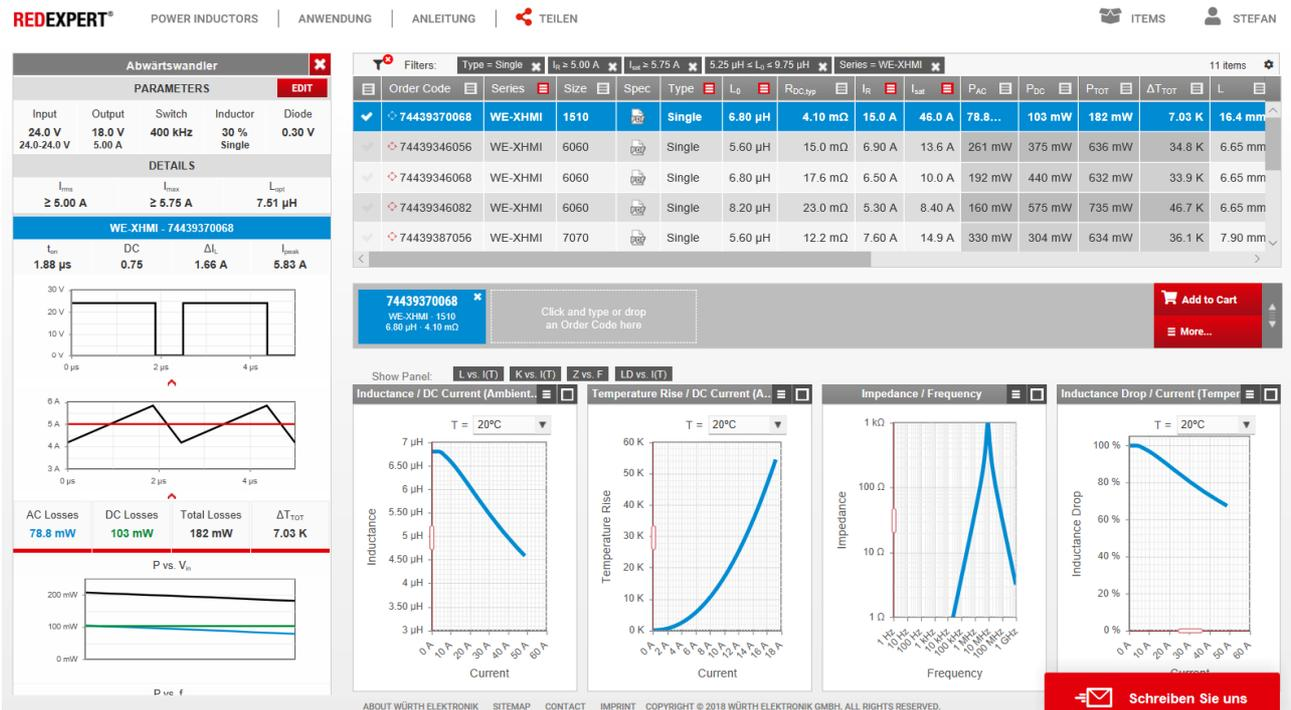
Figure 5: REDEXPERT simulation (buck operation) of WE-XHMI 74439370068.
