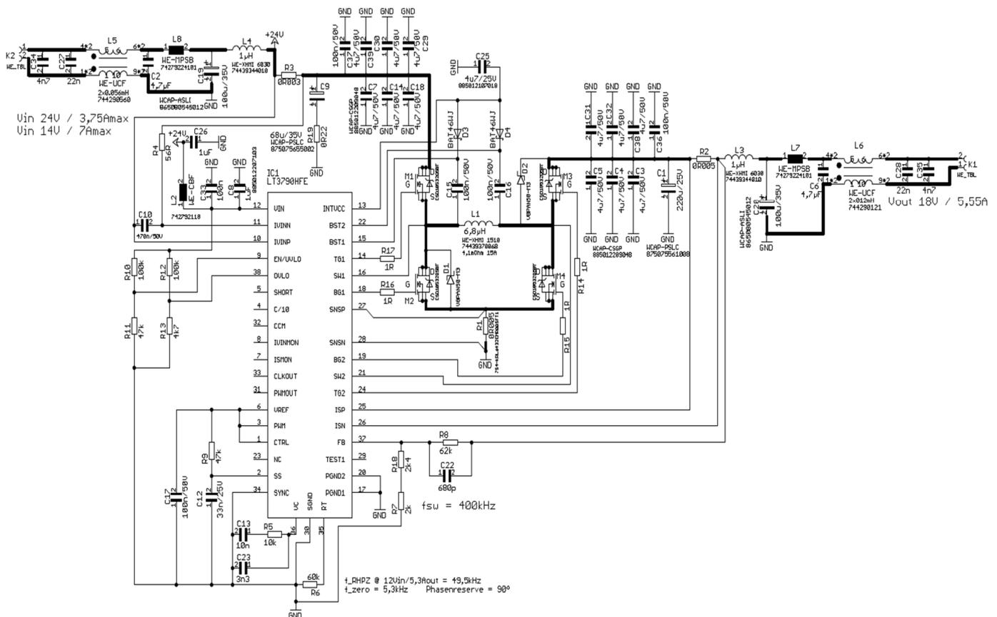
Figure 7: Circuit diagram of 100 W buck-boost converter, including all filter components.
