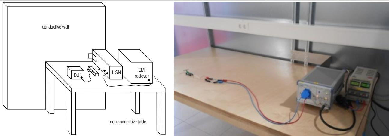
Figure 5: Setup of the EMC measurement according to CISPR 35
