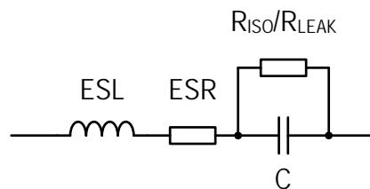
Figure 1: Equivalent circuit diagram of a real capacitor
