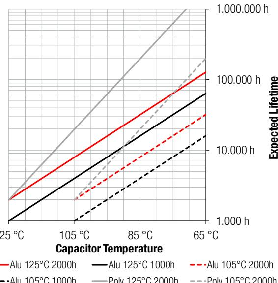
Figure 15: Overview of the expected lifetime of aluminum and aluminum polymer capacitors
