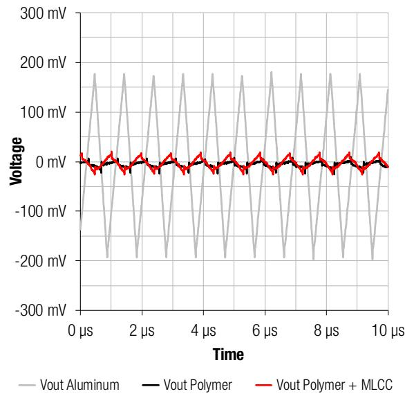
**Figure 14: Measurement of ripple voltage using an aluminum polymer capacitor and an MLCC**
