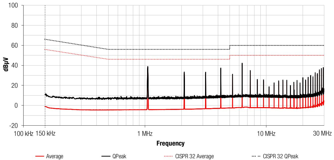
Figure 10: EMC measurement with input filter and aluminum polymer capacitor C<sub>1</sub>
