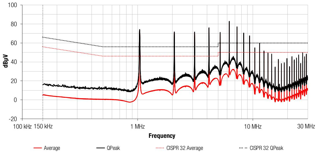
**Figure 8: EMC measurement with an aluminum polymer capacitor as input capacitor C<sub>1</sub>**
