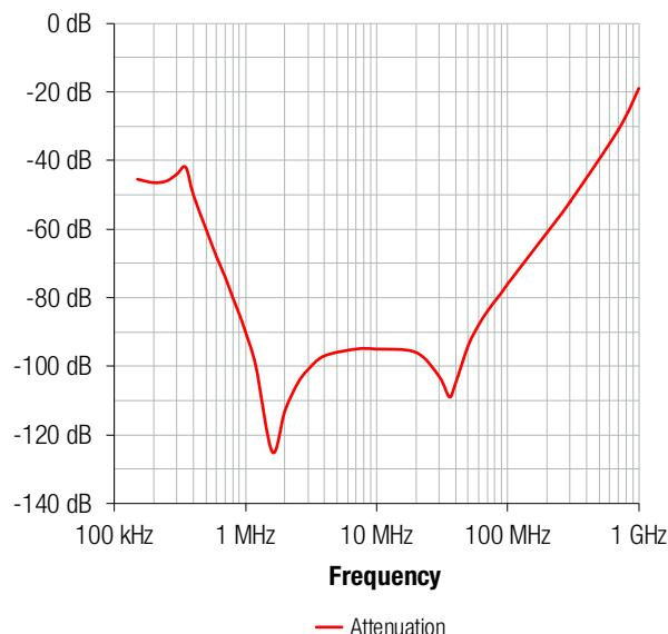
**Figure 9: Built-in input filter with simulated filter performance**
