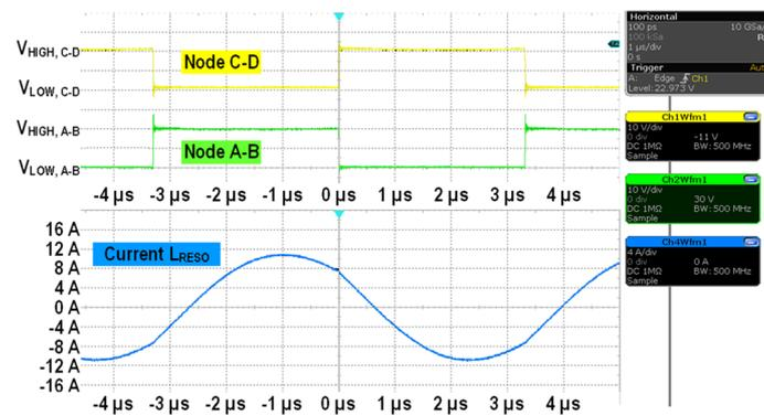
Figure 6: Oscillogram drain signals A-B, C-D and coil current
