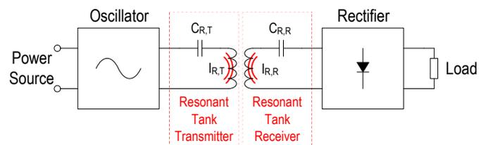
Figure 3: Principle of resonant inductive energy transfer
