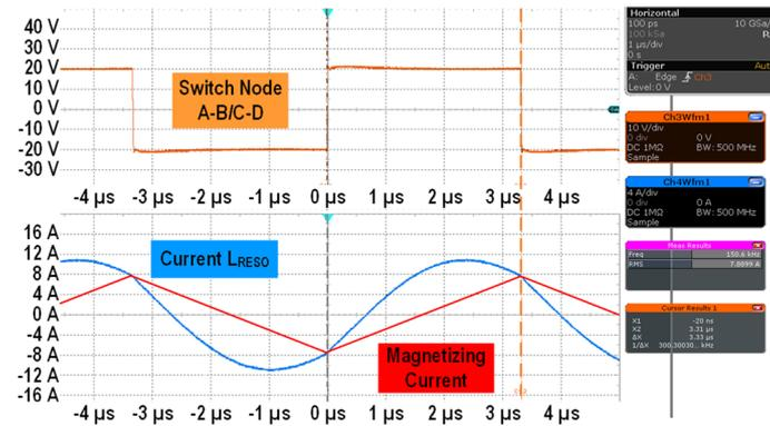
**Figure 8: Switching frequency and magnetising current**
