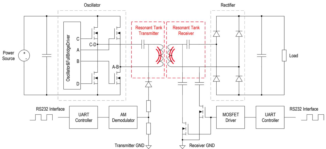
**Figure 10: Principle of data transmission from receiver to transmitter**
