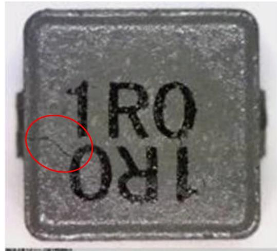
**Figure 5: Crack line on surface not acceptable**
