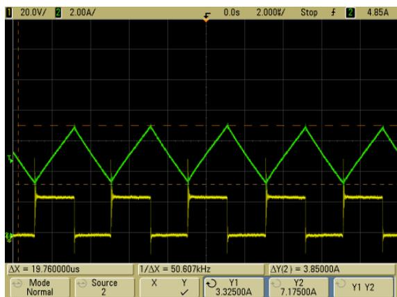
Figure 13: Inductor current and switching Voltage with 15% chipping on the Inductor body
