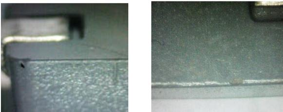
Figure 9: Acceptable chip off at surface junction
