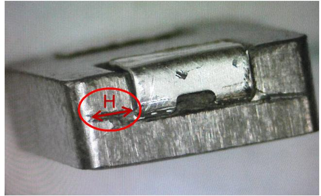
Figure 1: Hairline crack and definition of H
