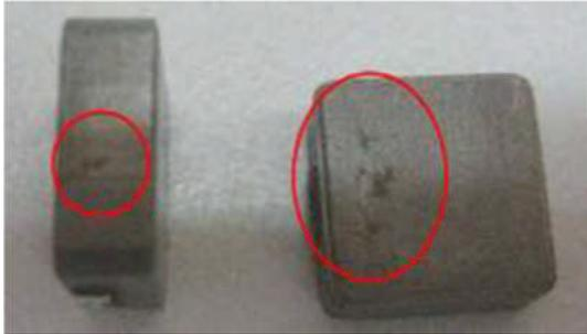
Figure 7: Oxidation on the core, rejected
