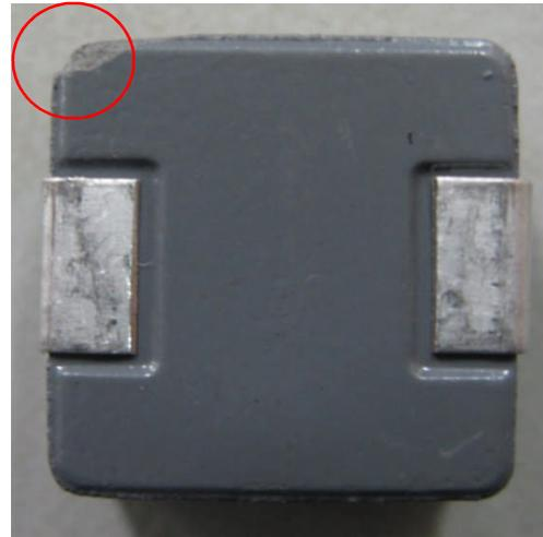
Figure 10: Rejected chip off at three surface junctions
