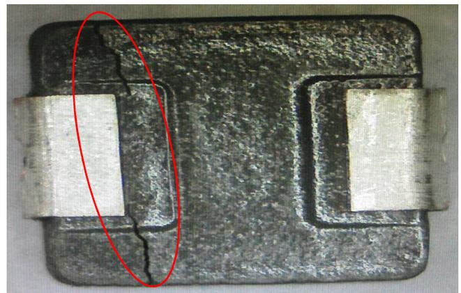
**Figure 6: Crack at the bottom, >2mm not acceptable**
