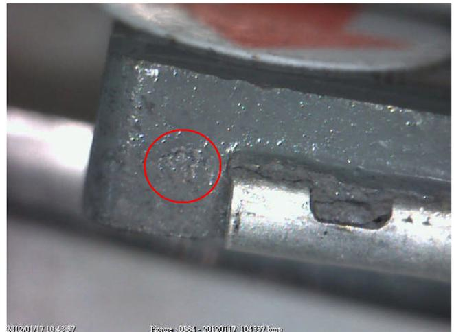
Figure 2: Acceptable minor crack on left side of terminal
