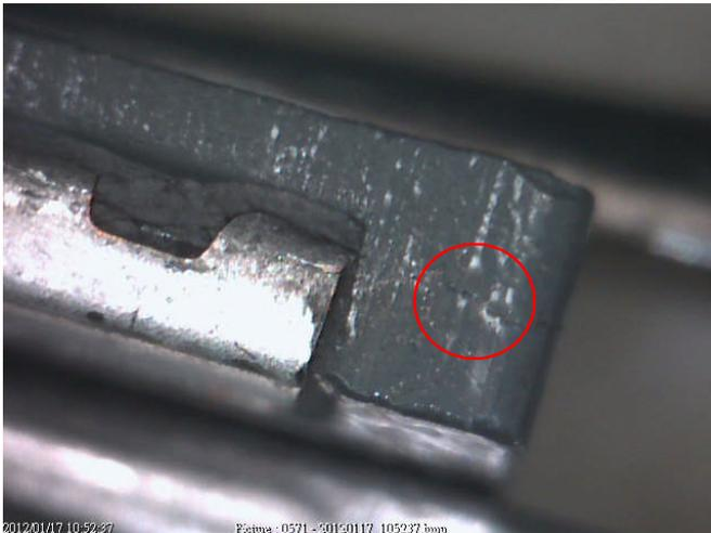
**Figure 3: Acceptable moderate crack on right side of terminal**
