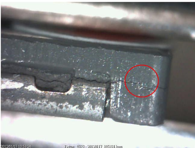
**Figure 4: Acceptable major crack on right side of terminal**
