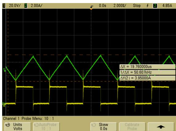
Figure 12: Inductor current and switching voltage with no irregularities on the inductor body
