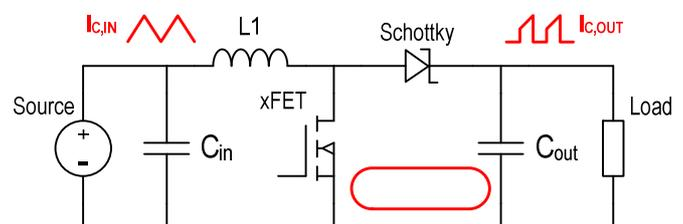
Figure 6: critical current loop boost converter
