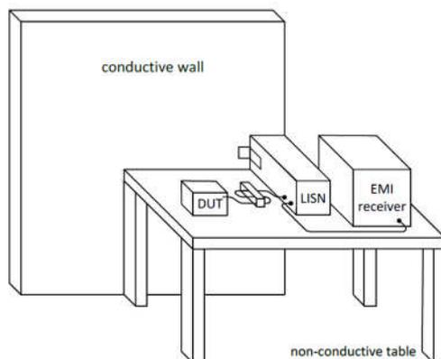
Figure 1: Test set-up for interfering voltage
