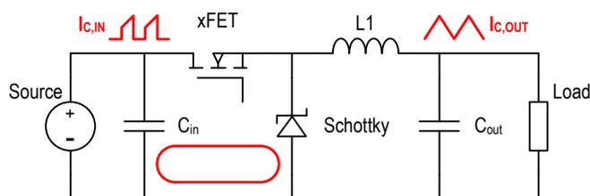
Figure 5: critical current loop buck converter
