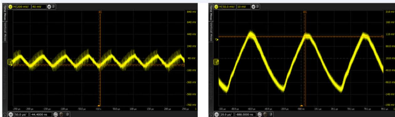
Output voltage (AC coupled) **200mV/Div**
