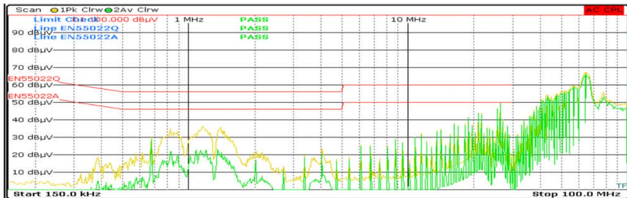
Figure 22: Measurement of the interference voltage of Design (1) at the **input** of the boost converter **with** LC filter (15  $\mu$ H / 10  $\mu$ F)
