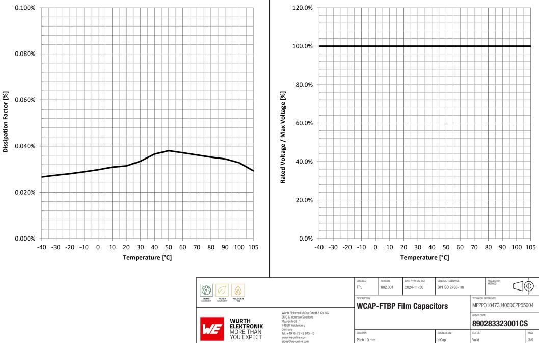
**Rated Voltage vs. Temperature:**
