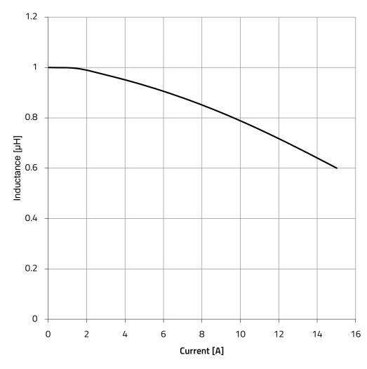
CHECKED REVISION DATE (YYYY-MM-DD) GENERAL TOLERANCE AdKa 003.001 2024-09-16 DIN ISO 2768-1m HALOGEN **WE-MAIA SMT Power Inductor** Würth Elektronik eiSos GmbH & Co. KG ORDER CODE EMC & Inductive Solutions **WURTH** Max-Eyth-Str. 1 78438357010 74638 Waldenburg **ELEKTRONIK** Germany MORE THAN YOU EXPECT SIZE/TYPE STATUS Tel. +49 (0) 79 42 945 - 0 BUSINESS UNIT PAGE www.we-online.com 2/8 4030 eiSos Valid eiSos@we-online.com
