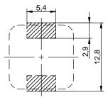
no sensitive traces underneath the component
