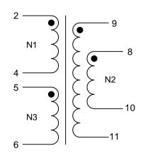
N2 denotes two windings connected in parallel. Terminals 8+9 and 10+11 must be tied as solder bridging is allowed.
