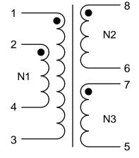
N1 denotes two windings connected in parallel. Terminals 1+2 and 3+4 must be tied as solder bridging is allowed.
