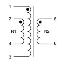
N1 denotes two windings connected in parallel. Terminals 1+2 and 3+4 must be tied as solder bridging is allowed.
