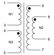
N2 denotes two windings connected in parallel. Terminals 6+7 and 8+9 must be tied as solder bridging is allowed.
