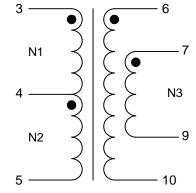
N3 denotes two windings connected in parallel. Terminals 6+7 and 9+10 must be tied as solder bridging is allowed.
