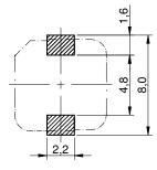
no sensitive traces underneath the component
