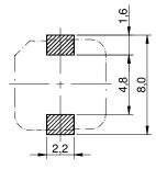
no sensitive traces underneath the component
