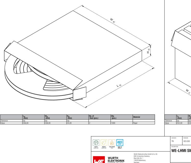
Qty. (pcs.) (mm) (mm) Material Inner Carton (pcs.) tvp typ. 354.00 348.00 4000 Paper DATE (YYYY-MM-DD) GENERAL TOLERANCE PROJECTION METHOD  $\oplus$ 2024-12-27 DIN ISO 2768-1m **WE-LHMI SMT Power Inductor** ORDER CODE 744373965056
