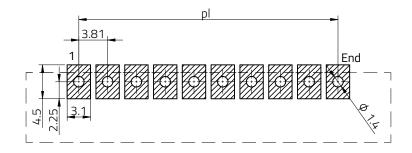
Stencil thickness: 120 µm
