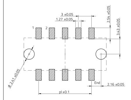
Max. Recommended PCB thickness: 1.6mm
