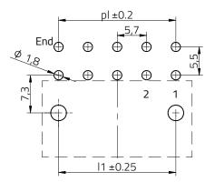
Recommended PCB layout thickness: 1.6 mm
