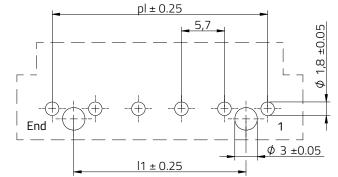
Recommended PCB Layout Thickness : 1.6 mm General tolerance ± 0.05 mm
