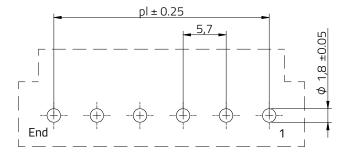
Recommended PCB Layout Thickness : 1.6 mm General Tolerance ± 0.05 mm
