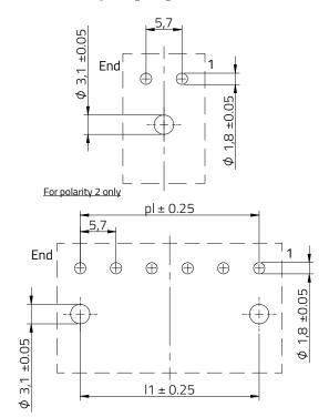
Recommended PCB Layout Thickness : 1.6 mm General Tolerance ± 0.05 mm
