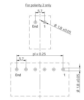
Recommended PCB Layout Thickness : 1.6 mm General tolerance ± 0.05 mm
